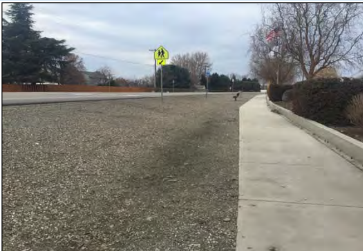
Runoff flows down slope to bus stop and sidewalk.
