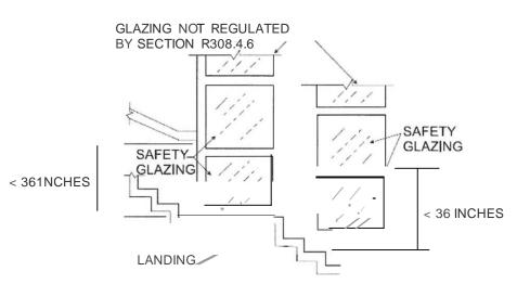
stairway where the glazing is less than 36 inches above the landing and within 60 inches horizontally of the bottom tread shall be considered a hazardous location. [IRC R308.4.7]
