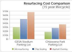
the cost savings are significant (microsurfacing costs as little as 20% of the cost of an overlay). While microsurfacing is typically done every 7-8 years (as compared to every 12-15 years for an overlay) the process extends the life of asphalt significantly, resulting in savings of more than 60% over the useful life of the pavement.
