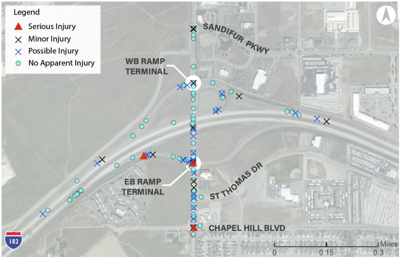
FIGURE 11: CRASH SEVERITY FOR ALL COLLISIONS ANALYZED ALONG STUDY CORRIDOR.
