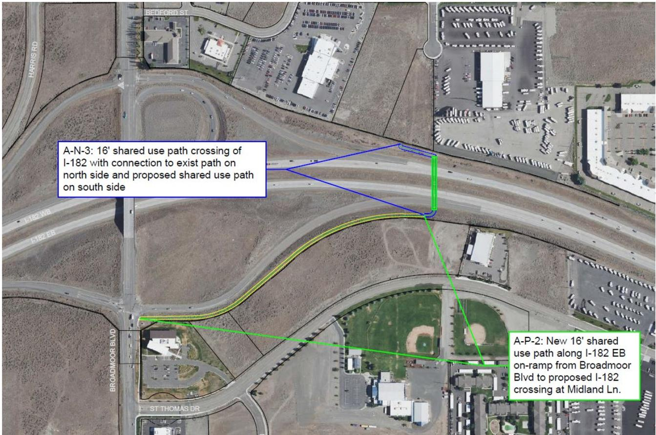
**FIGURE 32: ALTERNATIVES A-N-3 AND A-P-1 CONCEPTUAL LAYOUTS**
