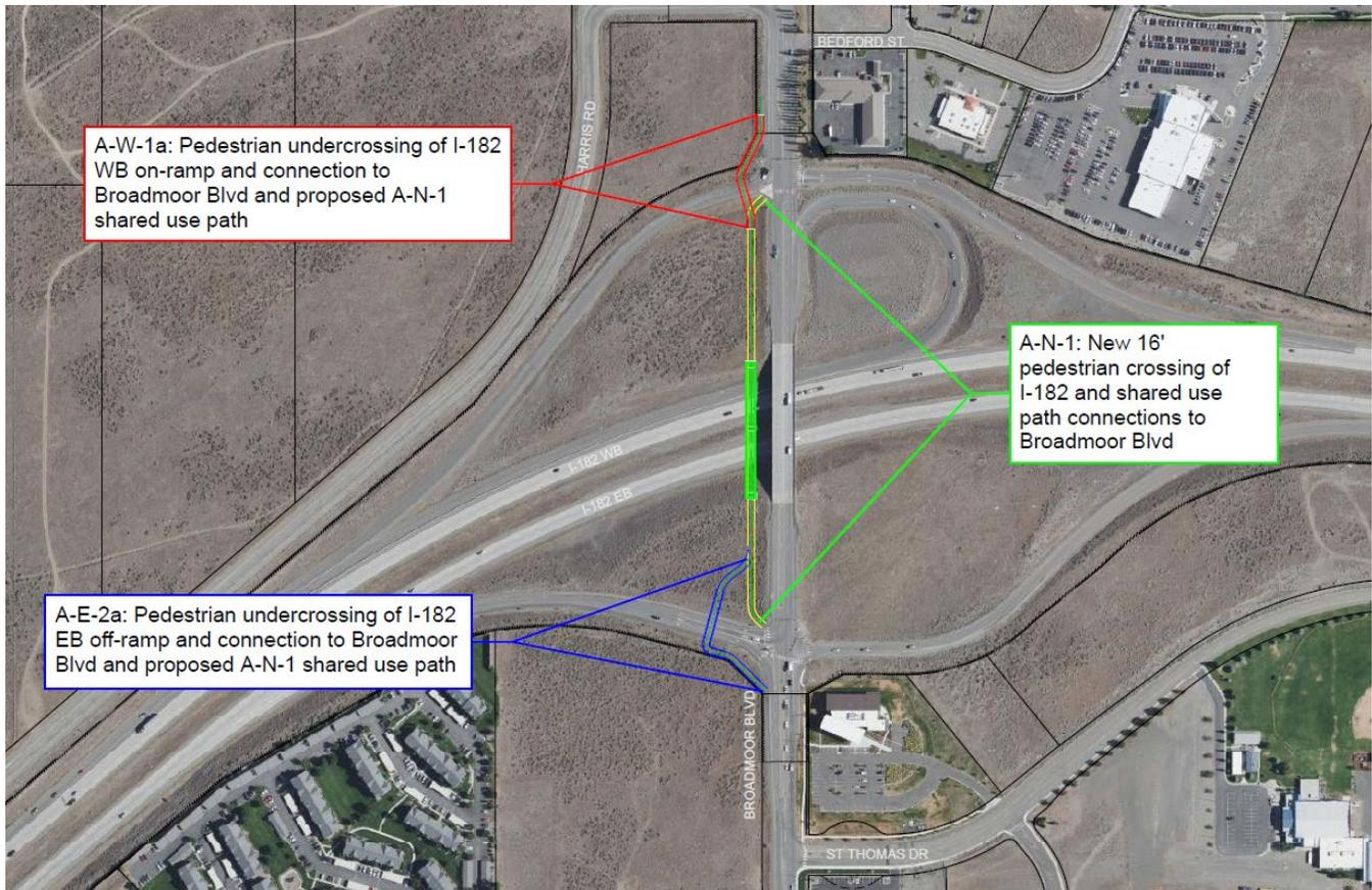
**FIGURE 30: ALTERNATIVES A-N-1, A-W-1A, AND A-E-2A CONCEPTUAL LAYOUTS**
