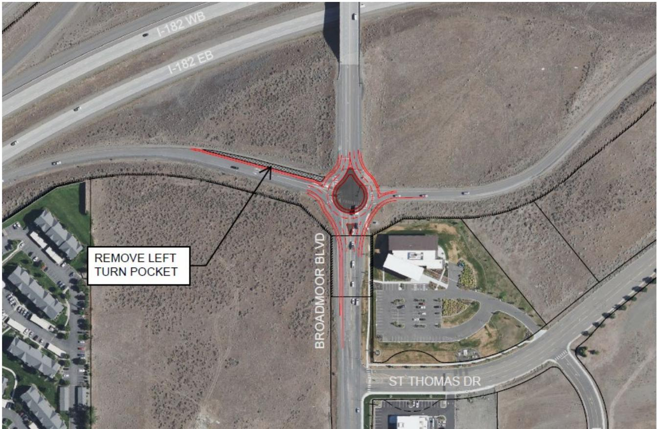
**FIGURE 28: ALTERNATIVE E-R-2 (ROUNDBOUT) CONCEPTUAL LAYOUT**
