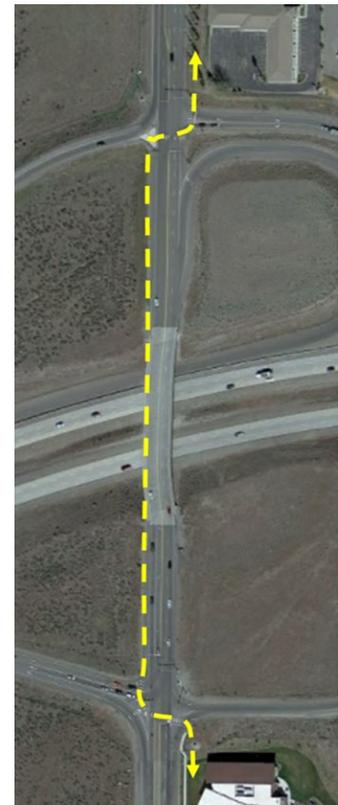
**FIGURE 10: PROTECTED PEDESTRIAN ROUTE THRU INTERCHANGE**
