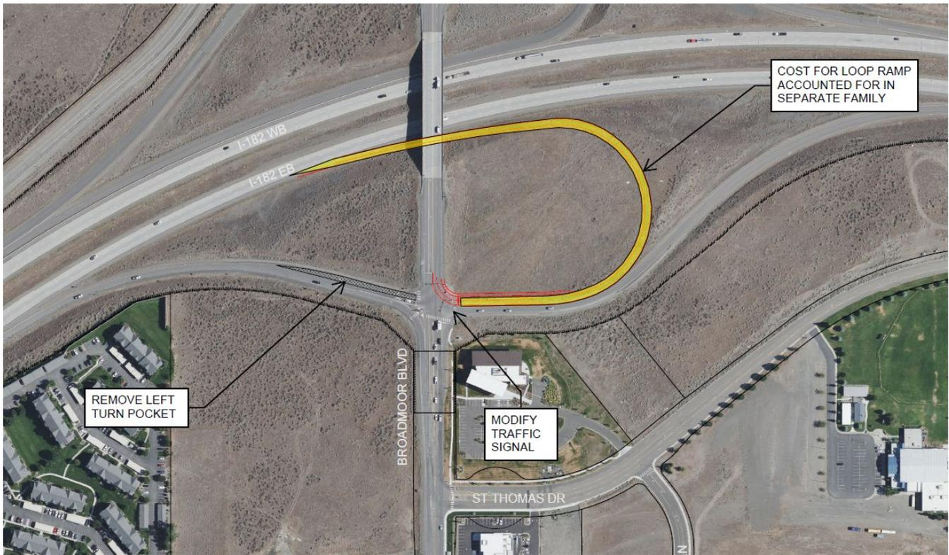
**FIGURE 29: ALTERNATIVE E-S-1 (SIGNAL + LOOP RAMP) CONCEPTUAL LAYOUT**
