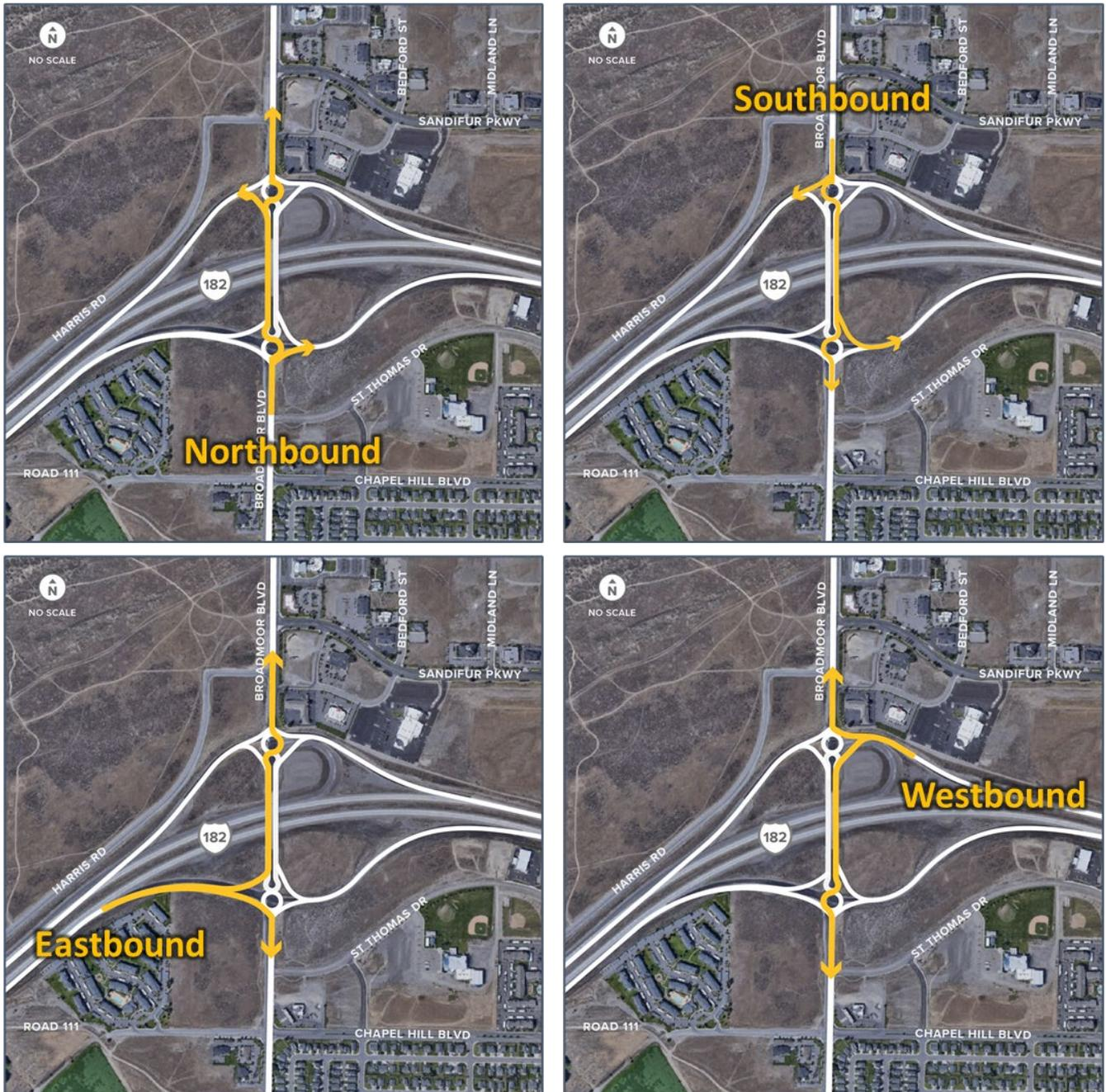
**FIGURE 36: DDI WITH ROUNDABOUTS CIRCULATION DIAGRAM**
