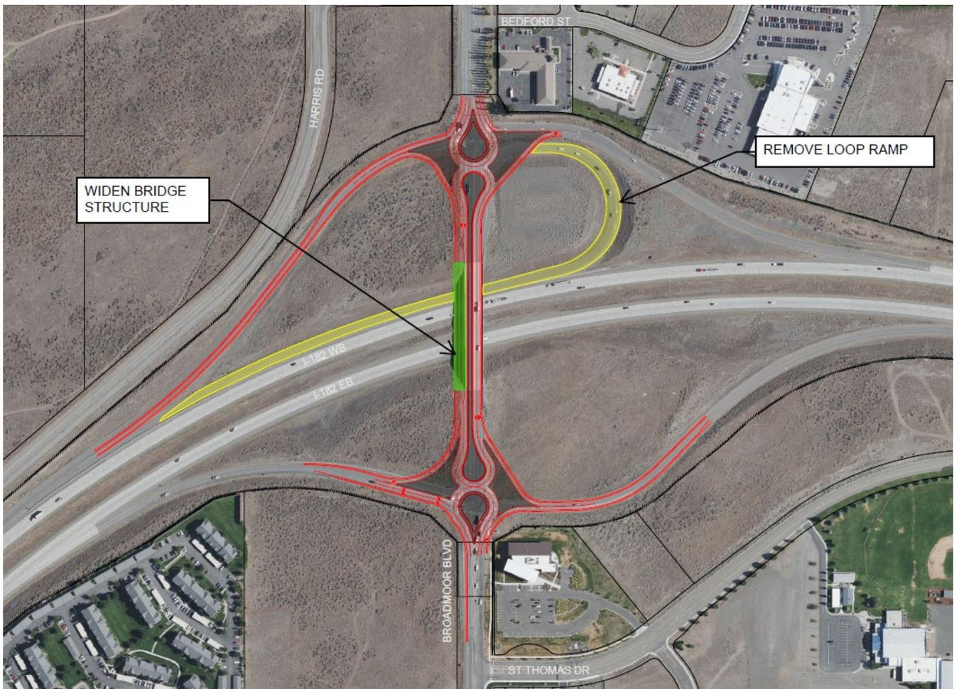
**FIGURE 35: ALTERNATIVE C-P-3 (DDI WITH ROUNDABOUTS) CONCEPTUAL LAYOUT**
