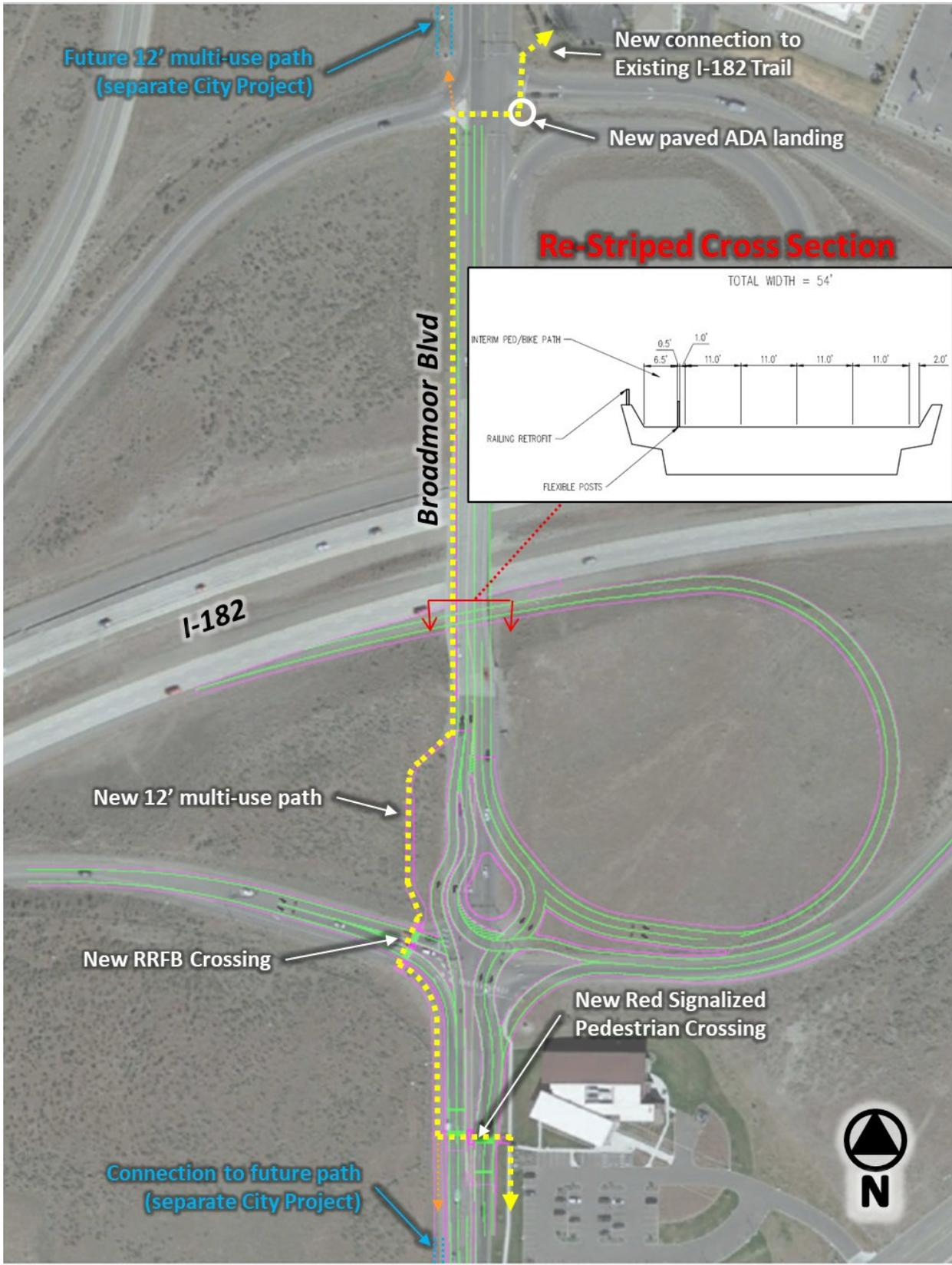
**FIGURE 40: PHASE 1A ACTIVE TRANSPORTATION ELEMENTS**
