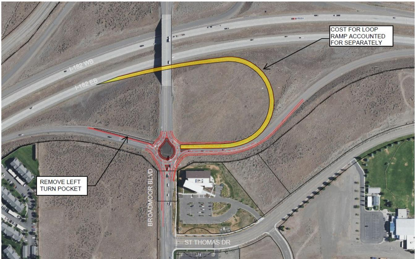
**FIGURE 27: ALTERNATIVE E-R-1 (ROUNDAABOUT + LOOP RAMP) CONCEPTUAL LAYOUT**
