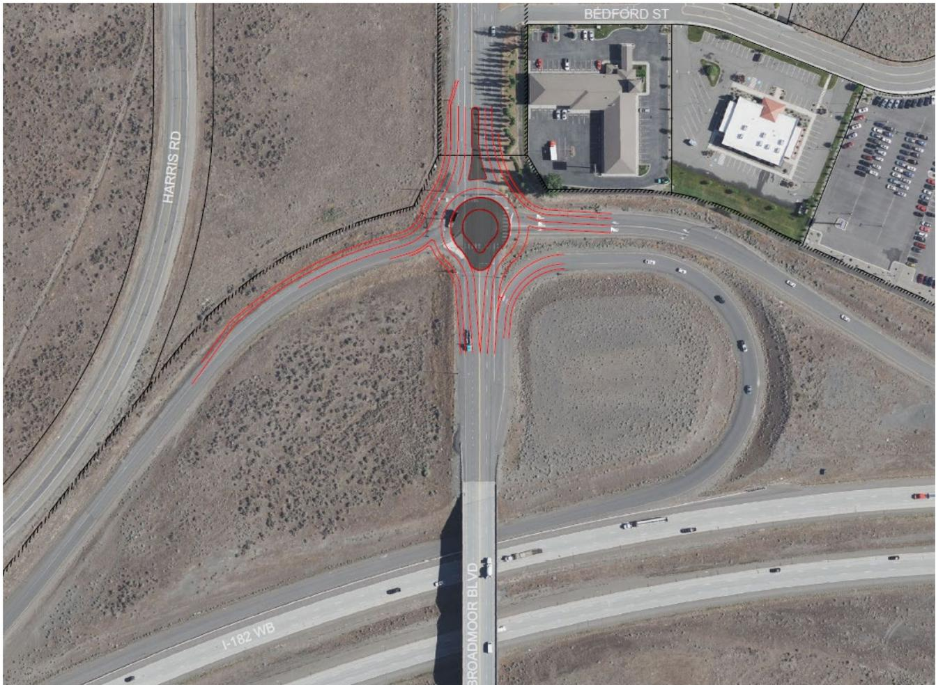
**FIGURE 26: ALTERNATIVE W-R-1 (ROUNDAABOUT) CONCEPTUAL LAYOUT**
