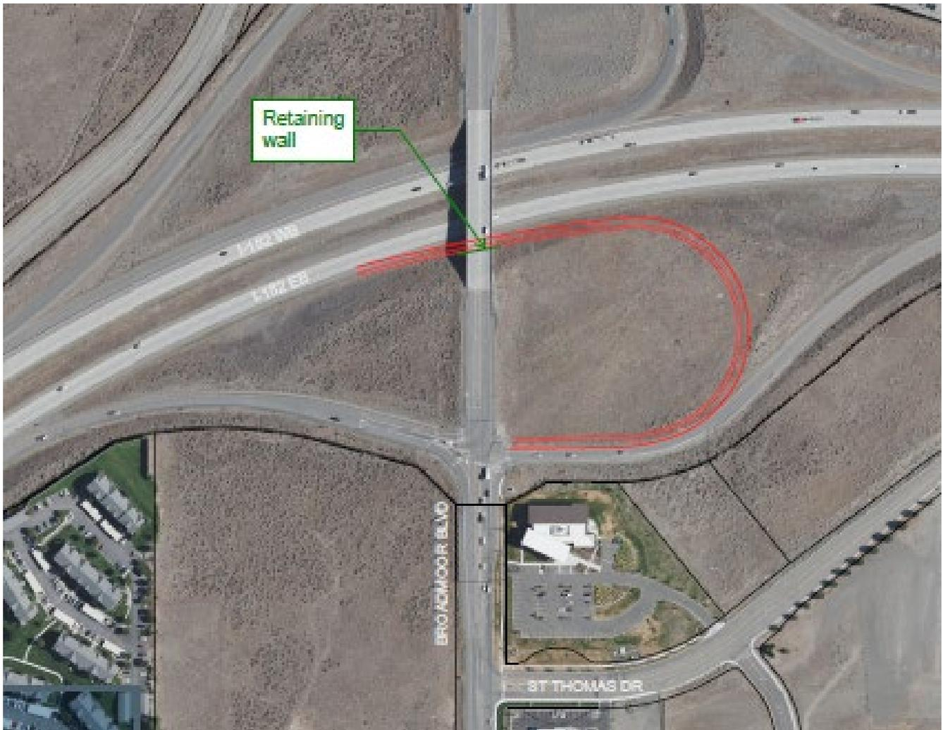
**FIGURE 21: ALTERNATIVE F-E-1 (LOOP RAMP) CONCEPTUAL LAYOUT**
